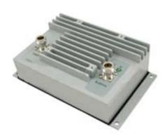
By directional amplifiers are compatible with 900 MHz wireless LAN equipment including the new generation 2.75 Mbit CCK (Complementary Code Keying) spread spectrum radios. The active power control circuit automatically adjusts the amplifier's gain to provide a constant output power regardless of cable length.
