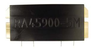
The new linear amplifier for UHF band is excellent design made for special applications, lab testing, digital and analog RF applications. This board requires 12 VDC / 1.5A. The minimum driving input is 10 mW; required RF input is 25 mW. Rated output RF power is 5 W.
