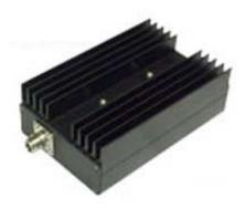
Video transmitter LX-430 is a high power unit made for long range application. This audio video transmitter has 12 selectable channels in UHF band. It has over 10 W RF power /50 ohms. This transmitter requires 12 V DC power / 4A.
