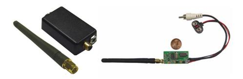
This small video transmitter for UHF is an excellent solution for video surveillance or experiments. The transmitter KX-900D is a 12 channels unit. It has 80 mW RF power. Dimensions: 2.4" X 1.5 "X 0.7". This transmitter sends a perfect color or B&W image to 900 MHz receiver including sound portion as well. Recommended receiver is M-808.
