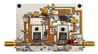
The new linear amplifier for UHF band is excellent design made for special applications, lab testing, digital and analog RF and TV applications. This board requires 12 VDC / 1.5 A. Amplifier covers full frequency range from 10 MHz-800 MHz. The minimum driving input is 10 mW; required RF input is 20-50 mW. Rated output RF power is 5 W, max 10 W/15V. Dimensions: 2.97" X 2.15"
